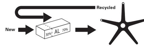
Recycling begins with AirPad well before production: as far as possible materials are used that have a high recycled content. Literally, the base of your current swivel chair is made out of the aluminium of the base of your disassembled old swivel chair and can be processed in the future to form the base of your new swivel chair.
